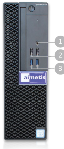
1. Universal audio jack | 2. USB 2.0 ports (1 with PowerShare) | 3. USB 3.0 ports | 4. Natively supports 3 digital video outputs (DP, DP and HDMI) | 5. Serial port | 6. More USB 3.0 ports | 7. USB 2.0 with smart power on | 8. PSU | 9. Security slot
