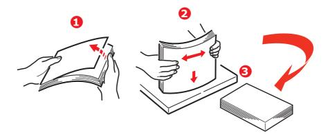
**3**. Load paper (letter headed paper face down and top edge towards the front of the printer), as shown.
