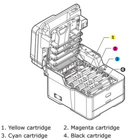
(a) Slide the coloured release collar on the cartridge to be replaced fully towards the right hand side of the printer.
