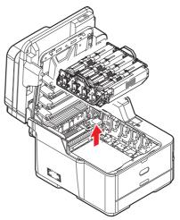
**5.** Put the assembly down gently onto a piece of paper to prevent toner from marking your furniture and to avoid damaging the green drum surface, and cover.
