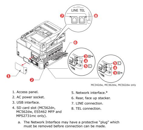
When the rear paper stacker is folded down paper exits the printer through the rear of the printer and is stacked here face up. This is mainly used for heavy print media. When used in conjunction with the multi purpose feed tray, the paper path through the printer is essentially straight. This avoids bending the paper around curves in the paper path and enables feeding of up to 220g/m<sup>2</sup> media.
