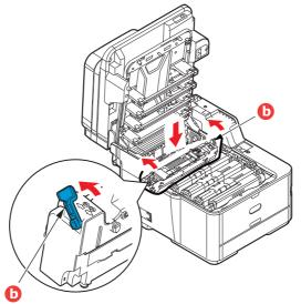
**10**. Close the top cover and press down firmly so that the cover latches closed.
