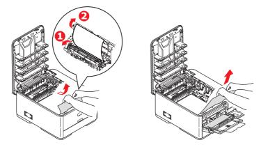
(b) To remove a sheet from the central area of the belt (b), carefully separate the sheet from the belt surface and withdraw the sheet.
