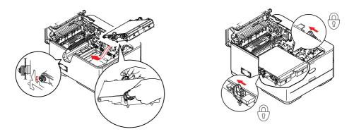
**8**. Push the locking levers towards the rear of the machine. This will secure the belt unit in place.
