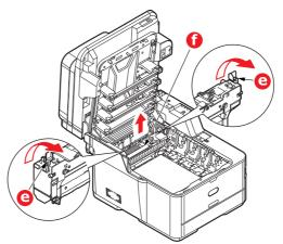
(e) Press release lever (g) and pull the trapped paper from the fuser.
