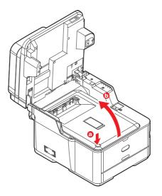
**3**. Identify the fuser handle (a) on the top of the fuser unit.
