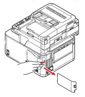
**3**. Turn locking screw (a) anti-clockwise and remove the inner access cover (b). Place it safely to one side.
