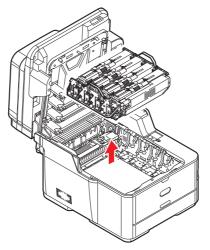
4. Place the assembly in a safe place away from direct sources of heat and light.
