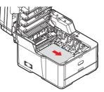
(c) To remove a sheet just entering the fuser (c), separate the trailing edge of the sheet from the belt, push the fuser pressure release lever (d) towards the front and down to release the fuser's grip on the sheet, and withdraw the sheet
