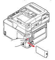
**3**. Turn locking screw (a) anti-clockwise and remove the inner access cover (b). Place it safely to one side.
