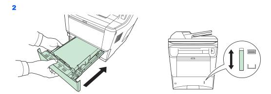
There is a paper gauge on the right side of the front of the paper cassette to indicate the remaining paper supply. When paper is exhausted, the pointer will go down to the level of <code>\_\_\_</code> (empty).
