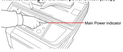
Press the Power key. The Power key light will go out, and the Main Power indicator will light up.
