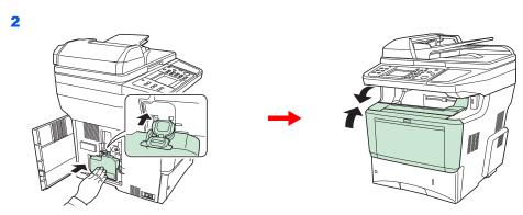
After replacing the toner containers and the waste toner box, clean the internal parts. For instructions, refer to Cleaning on page 10-7.
