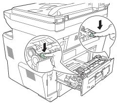
Press the two envelope switches (green) to change the paper feed mode to envelope mode.
