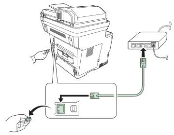
2 Connect the other end of the cable to the hub.
