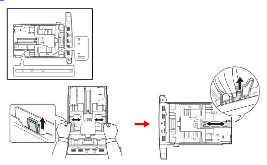
Adjust the cassette size to reflect the size of paper being loaded. Paper sizes are marked on the cassette.
