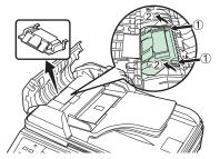
While pressing down on the hooks (x2) shown in the diagram, lift up and remove the separation pad.
