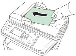
Put the side to be scanned (or the first side of two-sided originals) face-up. Slide the leading edge into the document processor as far as it will go.
