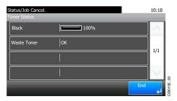
You can check the remaining amount of toner as one of 11 levels from 100 to 0%, and check the status of waste toner box.
