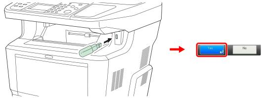
Plug the USB memory into the USB memory slot.
