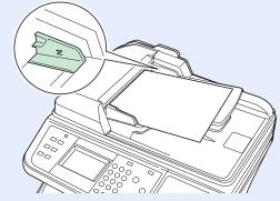
Confirm that the original width guides exactly fit the originals. If there is a gap, readjust the original width guides. The gap may cause the originals to jam.
