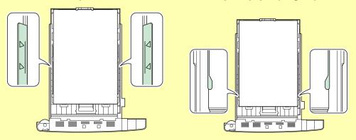
When loading the paper, keep the side that was closest the package seal facing up.
