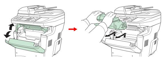
Open the top cover and front cover, and lift the developer unit together with the toner container out of the machine.
