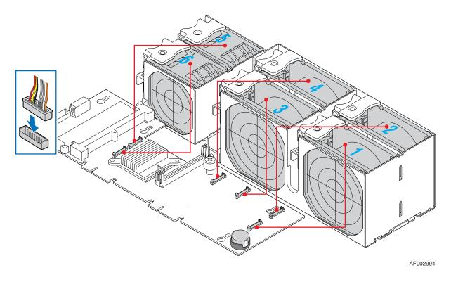
Figure 18. Redundant Fan Header Assignments on Midplane
