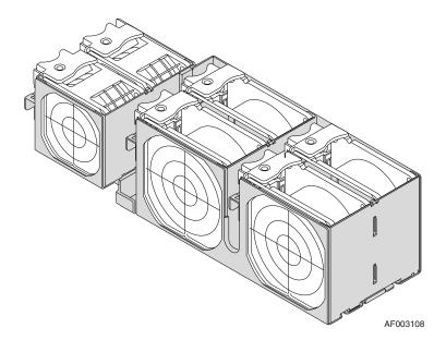
Figure 17. Fan Module Assembly
