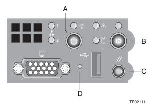
Figure 39. Control Panel Buttons
