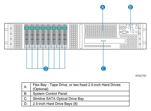
Figure 27. Flex bay for 3.5-inch Tape Drive or Two 2.5-inch HDDs (Front View)
