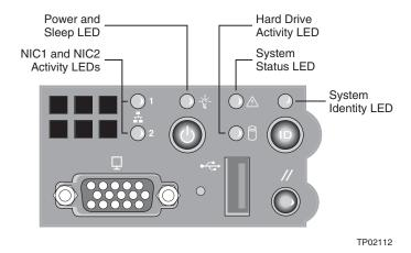
Figure 40. Control Panel LEDs
