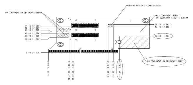
Figure 49. 2U Butterfly PCI-X/PCI Express\* Active Riser - Secondary Side
