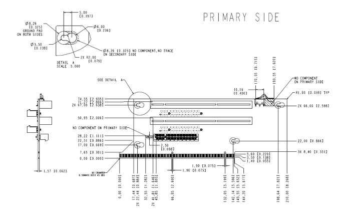
Figure 48. 2U Butterfly PCI-X/PCI Express\* Active Riser – Primary Side
