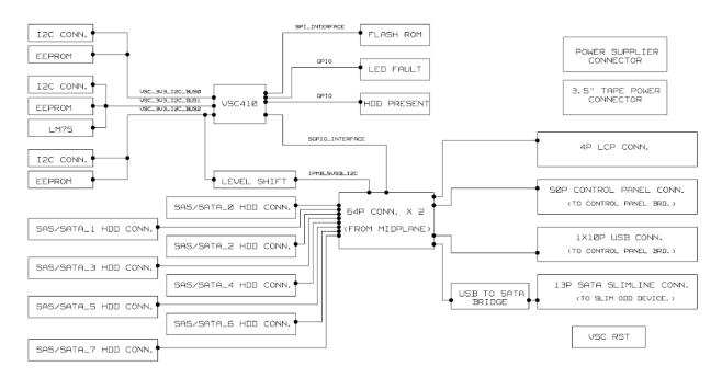
Figure 37. SAS/SATA Backplane Functional Block Diagram
