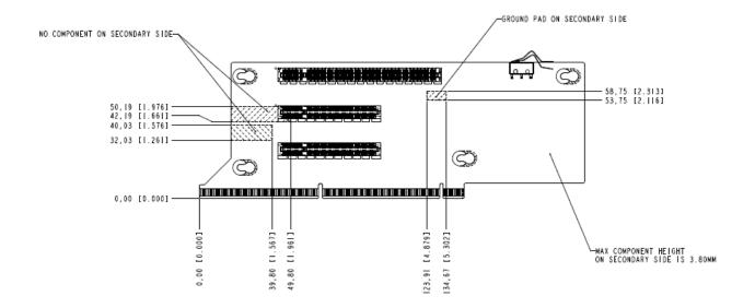
Figure 47. 2U PCI Express\* Passive Riser - Secondary Side
