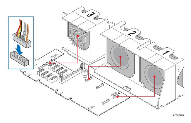
Figure 16. Non-redundant Fan Header Assignments on Midplane
