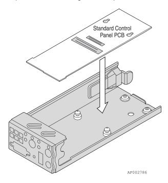
Figure 41. Standard Control Panel PCB
