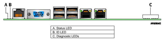
Figure 52. Diagnostic LED Placement Diagram
