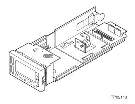
Figure 42. Intel<sup>®</sup> Local Control Panel Assembly Module
