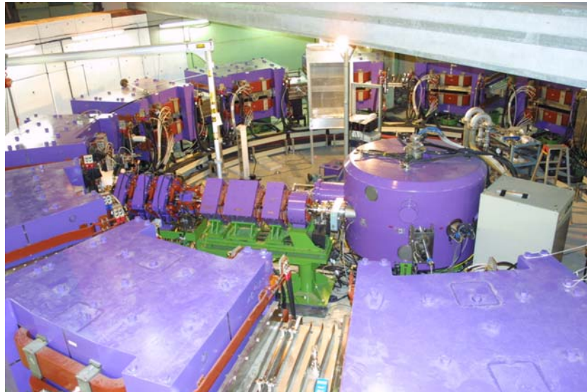
Figure 4: The 150 MeV scaling FFAG built at the KEK laboratory in Japan.
