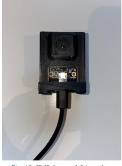
Fig. 10: FLIR Lepton 3.5 in casing.
