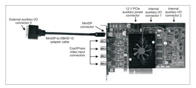
The MiniDP-to-DBHD-15 adapter cable connects to the MiniDP connector on the main bracket. The DBHD-15 connector at the end of this cable is called external auxiliary I/O connector 0.
