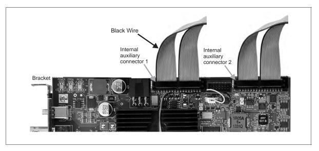
3. Slide the bracket of the cable adapter bracket into the opening at the back of the selected slot.
