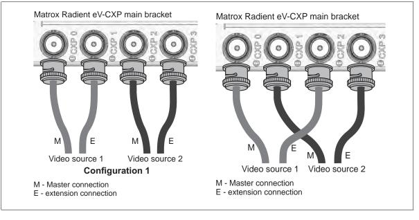
Matrox Radient eV-CXP communicates with the video sources to identify which video source is connected to which input connectors.
