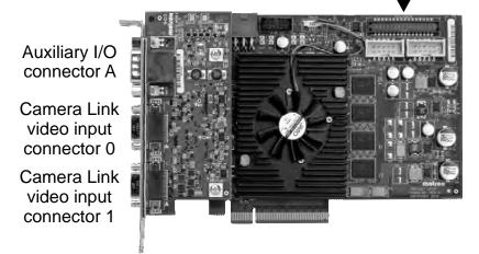
\*Use the 32-pin auxiliary I/O connector to connect to the DBHD-15 cable adapter bracket; Use the 10-pin auxiliary I/O connectors to connect to the DB-9 cable adapter bracket.
