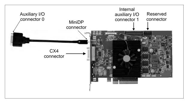
The MiniDP-to-DBHD-15 adapter cable connects to the MiniDP connector on the main bracket. The DBHD-15 connector at the end of this cable is called external auxiliary I/O connector 0.
