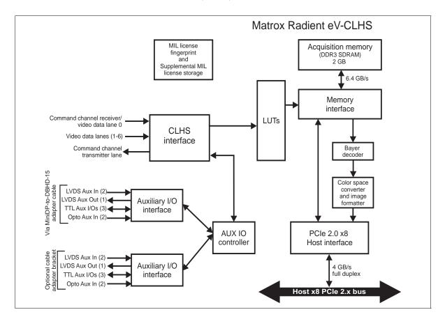
Matrox Radient eV-CLHS supports a single CLHS link to a video source that transmits data at 3.125 Gbits/sec per video data lane between the video source and frame grabber. A CLHS link contains all the connections and components to capture from one video source.
