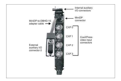
To access the signals of the internal auxiliary I/O connectors, you can install up to two cable adapter brackets. They each have two connectors that are named based on the internal auxiliary I/O connector to which their cable adapter bracket is attached.
