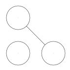
The amount that is chopped is by default equal to the radius of the circle. You can specify how much of the line is chopped, for use with other objects or text, by supplying either one or two values after the attribute. If a single value is given, then both ends of the line are chopped by that amount. If two values are given, the start of the line is chopped by the first amount and the end of the line chopped by the second amount.
