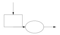
Note the short arrow, drawn from the box to the circle. What happened? The end point of the box was not on the right, but on the bottom, because the motion in effect where the box is drawn is down. Changing direction (right) affects only the direction in which the arrow is drawn; it does not change where the arrow begins. Thus, the arrow is drawn along the bottom line of the box.
