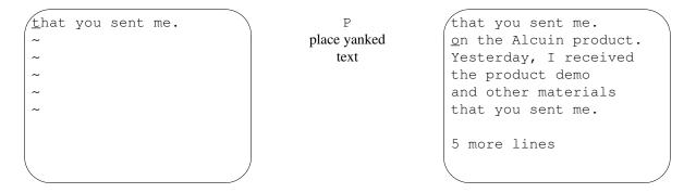
The yanked text will appear on the line below the cursor. Deleting uses the same buffer as yanking. Delete and put can be used in much the same way as yank and put. Each new deletion or yank replaces the previous contents of the yank buffer. As we'll see later, up to nine previous yanks or deletions can be recalled with put commands.
