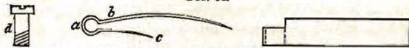
Fig. 34. Feed-finger spring , full size. a , eye; b , long branch; c , short branch; d , screw.
