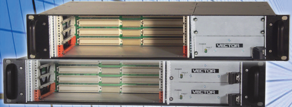
Series 815 Tower with 4 slot cPCI® or 5 slot VME 64x Backplane
