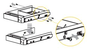
Step 2: Once the installation is completed, insert the tray back and fix it firmly in the proper place.
