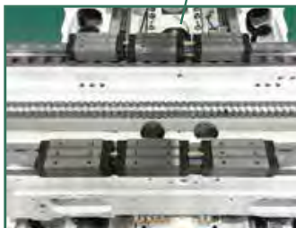
3-Block, Double Roller LM Guide System Ultra-super-high rigidity. Long term smooth motion operation.
