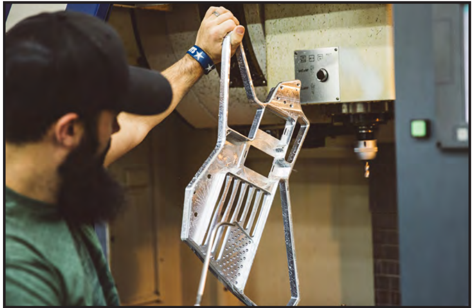
Drew Emory and his partner Myke Wilkerson are using the Emory tool shop as the manufacturing arm of their new venture "660 Guitars". Dynamic Motion technology is used to rapidly carve out 7.5 guitar bodies from 40 lb. aluminum billets.
