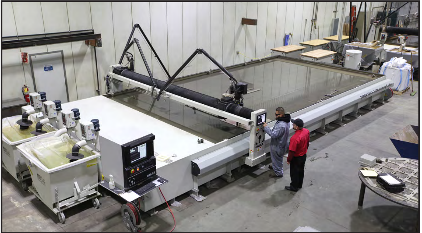
Petersen's OMAX 160X JetMachining Center provides a big cutting window of 13' x 26'.
