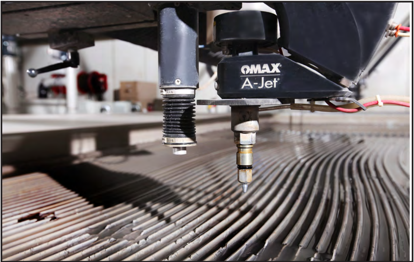
With its OMAX waterjet cutting capability, Petersen holds close to normal machining tolerances on fabricated parts as long as 14'.
