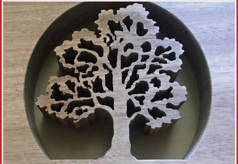
Top left - The ByJet Smart 3015 water head is a dual head system that doubles the parts output. Minimum separation is 8". Top right - An example of the precision capabilities of the water jet. The tree was cut out of a 3" deep piece of solid oak. Bottom - Kyle Standford runs and maintains the ByJet Smart 3015 water jet. Greg purchased it because it is a very sturdy and rugged machine. It has a concrete base for stability.
