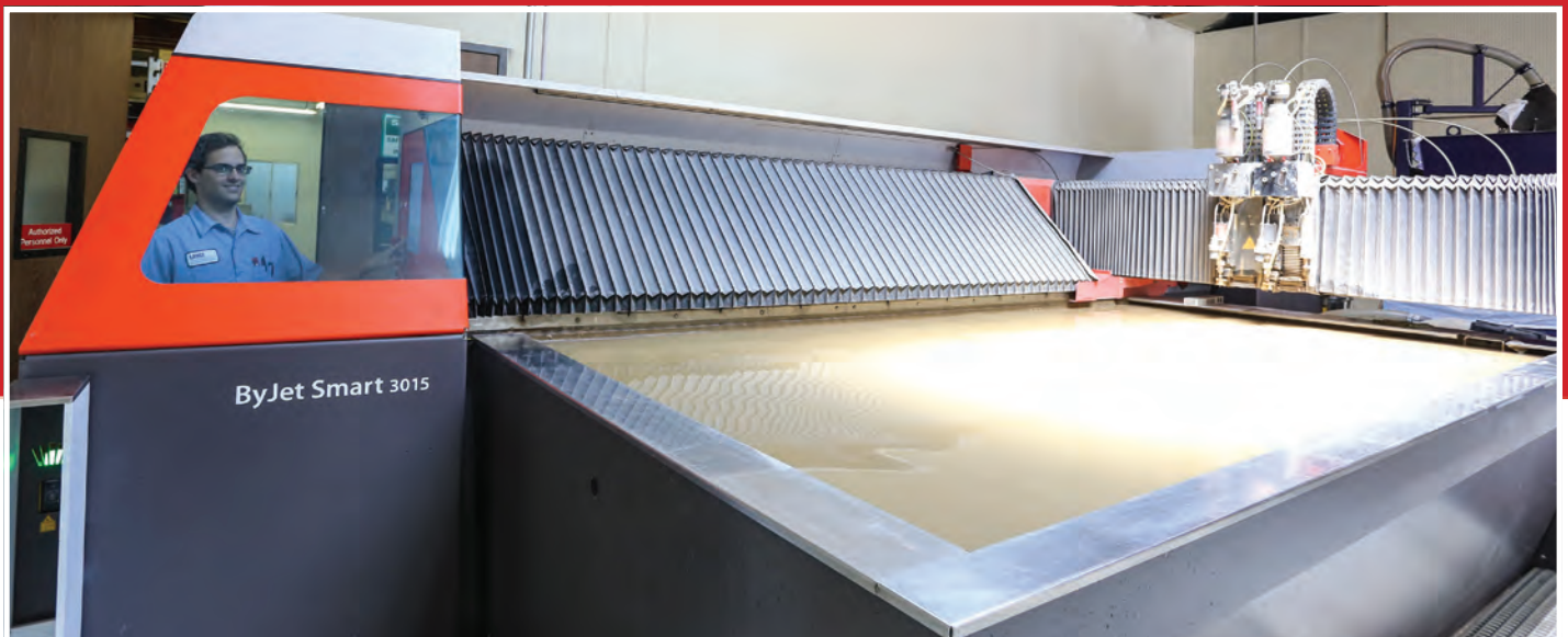
Top left - The ByJet Smart 3015 water head is a dual head system that doubles the parts output. Minimum separation is 8". Top right - An example of the precision capabilities of the water jet. The tree was cut out of a 3" deep piece of solid oak. Bottom - Kyle Standford runs and maintains the ByJet Smart 3015 water jet. Greg purchased it because it is a very sturdy and rugged machine. It has a concrete base for stability.
