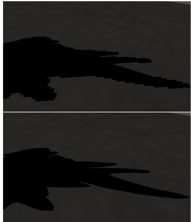
Figure 9: Aliasing in Shadow Mapping (top) and PSSM (bottom)
