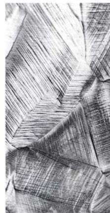
Slip lines on the surface of a polycrystalline specimen of copper
