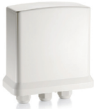
POR-1222 PoE+ Repeater, 2 Ports, Gigabit Ethernet, Outdoor, Cascadable
