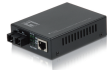
FVT-2201 10/100BASE-TX to 100BASE-FX SMF SC Converter, 20km
