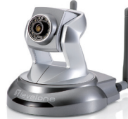
WCS-6050 PT Network Camera, 5-Megapixel, 150Mbps 802.11b/g/n, Day & Night, IR LEDs
