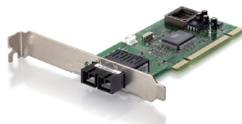
FNC-0104FX Fast Ethernet Fiber PCI Network Card, Multi-Mode, SC
