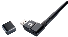
WUA-0614 Wireless USB Network Adapter, 150Mbps 802.11b/g/n, Nano
