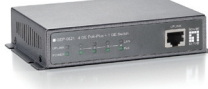
GEP-0521 5-Port Gigabit Ethernet PoE Switch, 120W, 802.3af/at PoE Plus, 4 PoE Outputs
