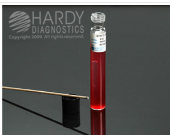
Figure 6. Red color development after the addition of zinc to a presumptive negative test result. ( http://hardydiagnostics.com/ )
