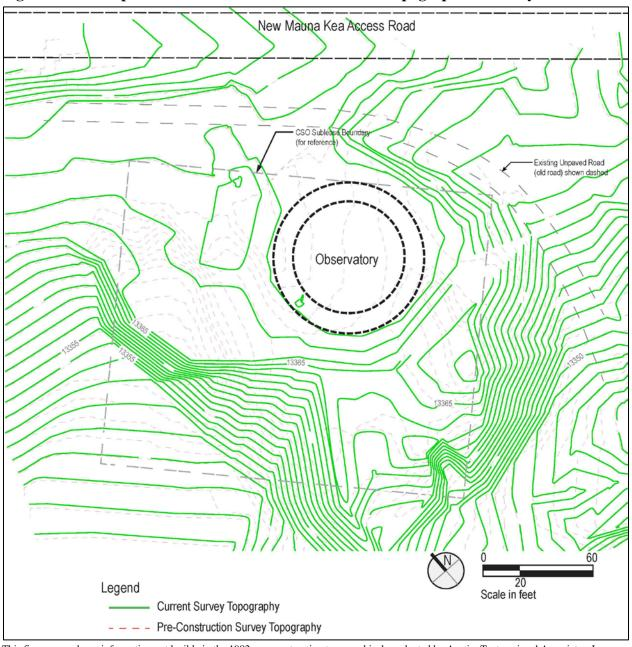
Figure 2.12 Comparison of Pre-Construction and 2016 Topographical Surveys
