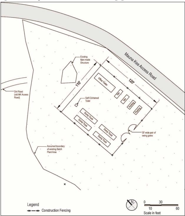
Figure 2.5 Conceptual Plan View of Deconstruction Staging Area 2
