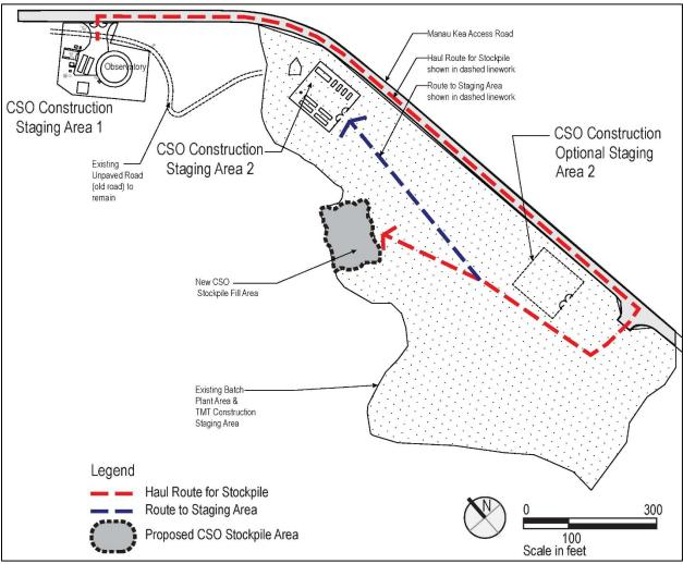
Figure 2.3 Conceptual Plan View of Overall Deconstruction Staging
