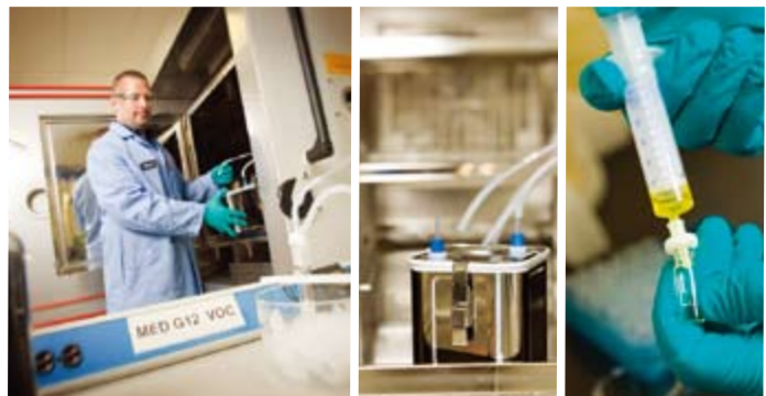
A Senior Technician in the Materials Engineering Department at the Toyota Technical Center performs a water extraction smell test to predict odor in the vehicle cabin.
