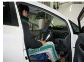
Rewriting the ABS program on a customer's Prius
