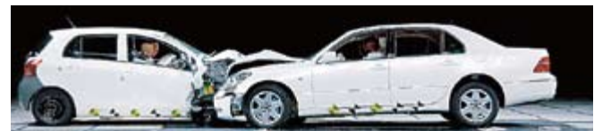
* Compatibility is a concept intended to assure mutual safety by securing the passive safety of lighter vehicles and reducing the harmful impact of heavier ones.
