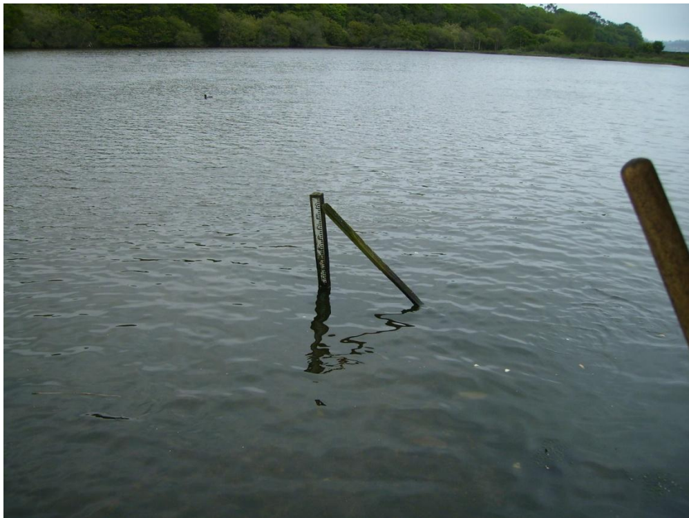
Figure 2. Staff gauge where water depth measurements were made in Cuskinny Lake during neap tides on 30 th April and during spring tides on 23 rd May 2012.
