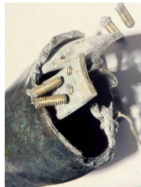
FIGURE 5.18. Brass plates and screws used in the reassembly of right arm
