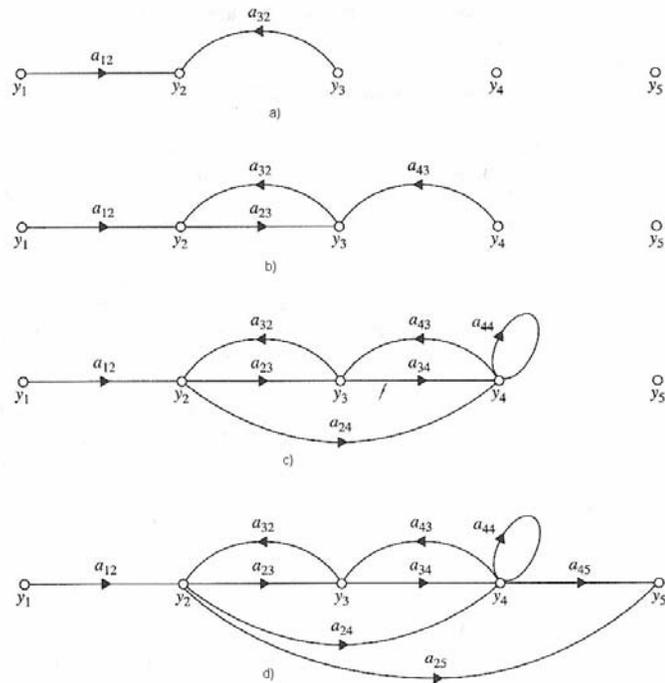
Figura 38. a)  $y_2 = a_{12}y_1 + a_{32}y_3$ ; b)  $y_2 = a_{12}y_1 + a_{32}y_3$  y  $y_3 = a_{23}y_2 + a_{43}y_4$ ; c)  $y_2 = a_{12}y_1 + a_{32}y_3$ ,  $y_3 = a_{23}y_2 + a_{43}y_4$  y  $y_4 = a_{24}y_2 + a_{34}y_3 + a_{44}y_4$ ; d) Diagrama de flujo completo.
