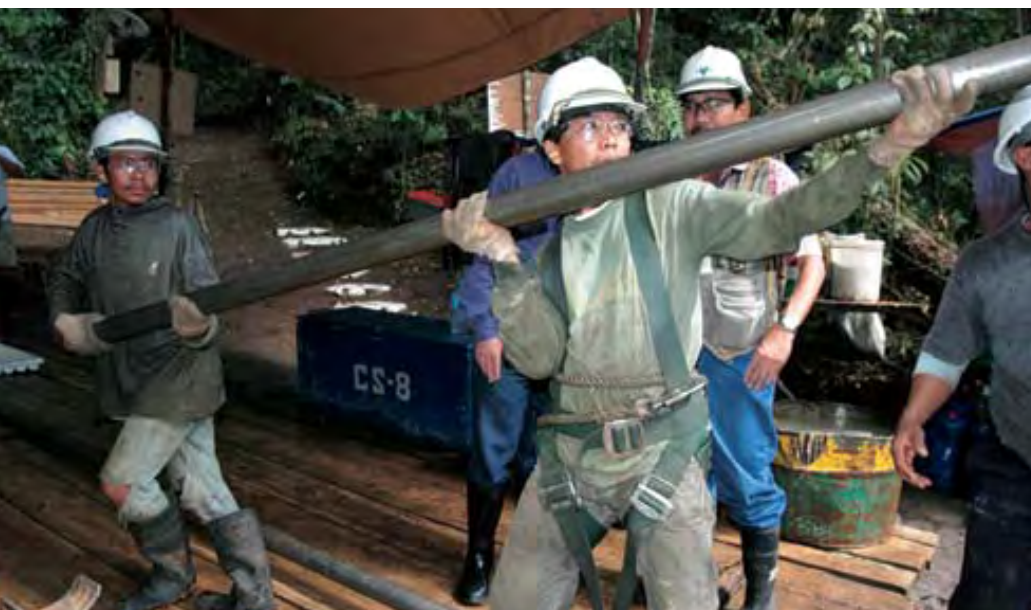
Changing the drill rod at the Tampakan exploration project, Philippines
