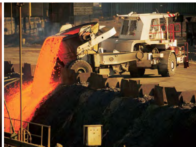
Waste is discharged to the cooling font at Altonorte smelter, Chile
