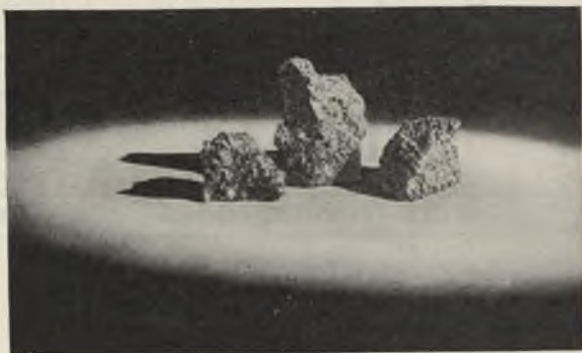
Norton Boron Carbide as it comes from the electric furnace (uncrushed)
