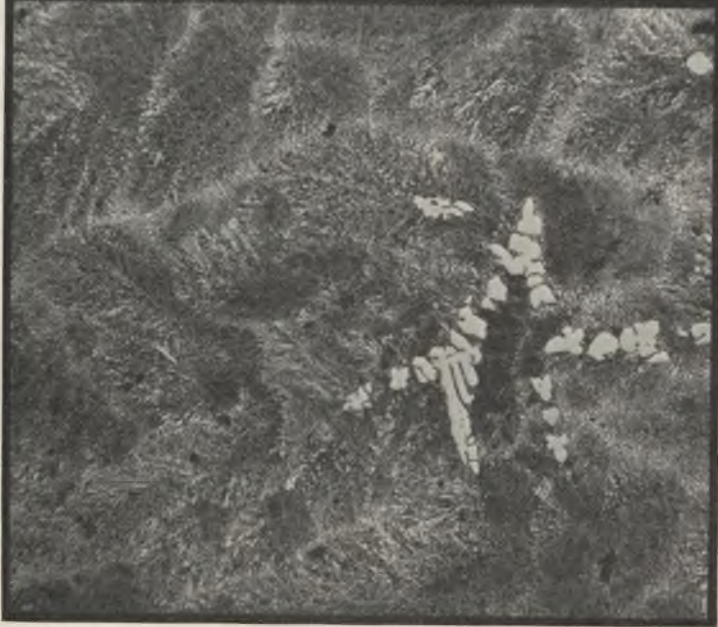
FIG. 7.—18.6% Cerium, As Cast. Etched in Citric Acid, Nitric Acid, and Glycerine. \times 150 . FIG. 8.—21.6% Cerium, As Cast. Etched in Citric Acid, Nitric Acid, and Glycerine. \times 150 .
