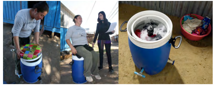
Figure 2. Techo staff field testing refined GiraDora clothes-washer/spin-dryer prototype by Alex Cabunoc and Ji A You, in campamento near Santiago, Chile.
