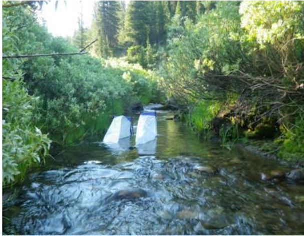
Figure 4. Drift nets used to quantify stream productivity through macroinvertebrate drift.
