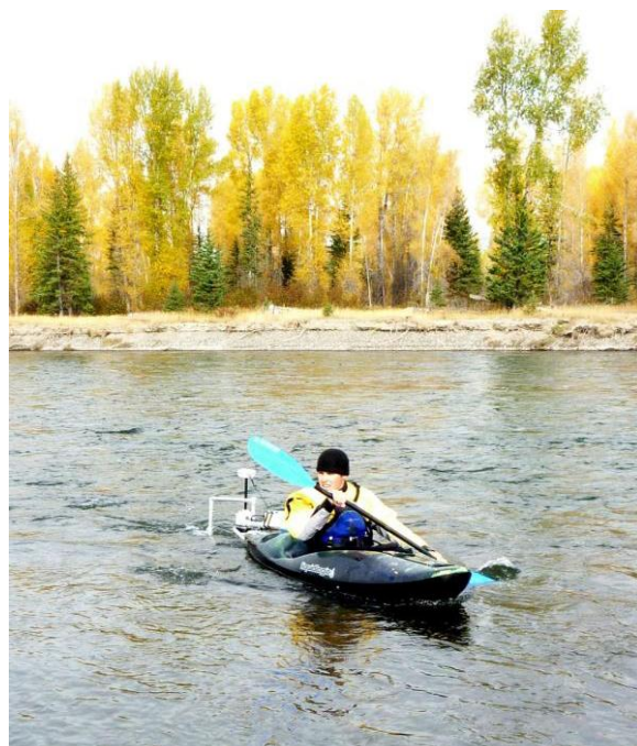
Figure 7. Flow velocities were measured with an acoustic Doppler current profiler (ADCP) deployed from a kayak, shown here during a September deployment intended to characterize the flow field at a lower discharge.
