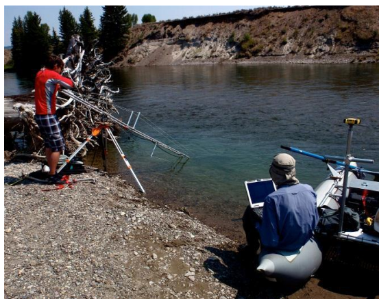
Figure 6. Measurement crane used to facilitate measurements of the downwelling radiant energy at different depths within the water column.
