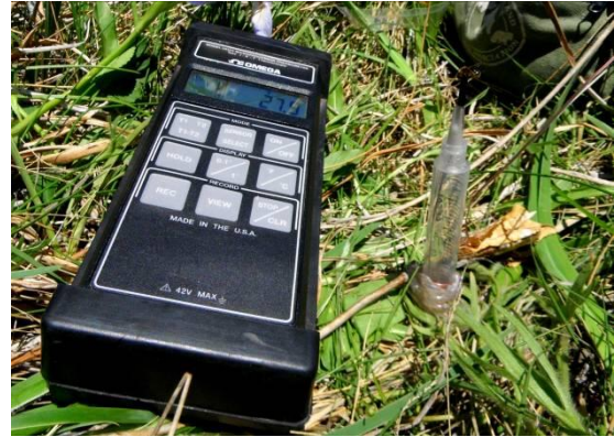
Figure 2. Operative temperatures were measured by inserting a fine thermocouple probe into a freshly killed bee.
