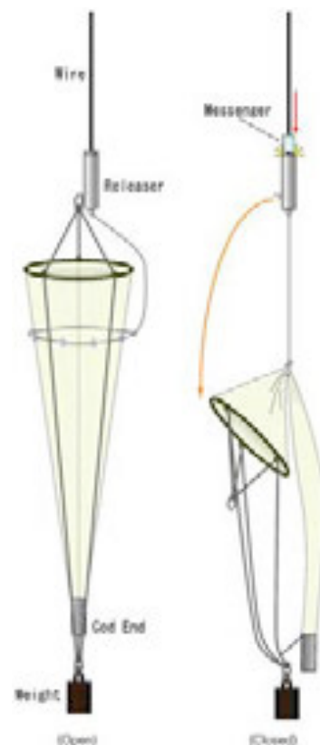
Fig.3-10-1 Schematic illustration of closing NORPAC net. Plankton net is open during towing (left), and closed at the top of the sampling depth range by deploying a messenger (right).
