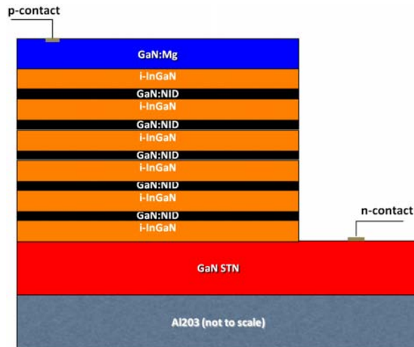
FIGURE 4.18 – Schéma de la structures pin "multicouche".
