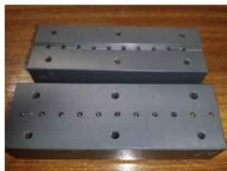
Fig. 6. Bloc of PVC to determine accurately the resistivity of samples at room temperature (0–50 °C).
