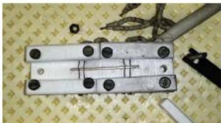
Fig. 7. Measurement of the resistivity: alumina pieces, sample, chromel and alumel wires.
