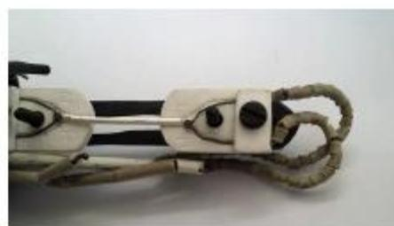
Fig. 5. Device for ATP measurement of AgNi sample.
