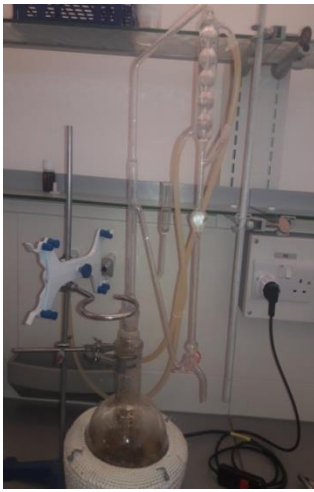
Figure 7: Images showing obtaining volatile oil of Chamomilla aurea
