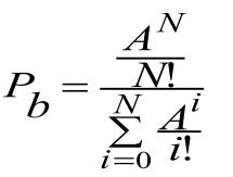
$P_{b} = \frac{\underline{A^{i}}}{\sum_{i=1}^{N} \underline{A^{i}}}$ where A = Offered Traffic N = Number of Servers (Lines) P\_{b} = Probability of Blocking
