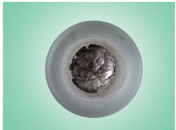
Fig. 9.10: Overtrituated mix sticks to be capsule which is difficult to remove
