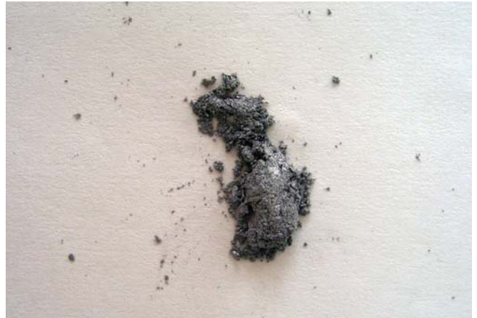
Fig. 9.9: Undertrituated amalgam mix appears dry and crumbled
