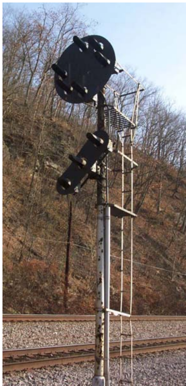
Figure 15. Color position signal with “yellow only” lower head
