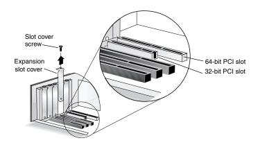
Computers may have vertical or horizontal expansion slots. Refer to your computer manual to locate the PCI slots. If your computer is a tower model, place it on its side to make it easier to install the Adaptec SCSI Card 29160LP.
