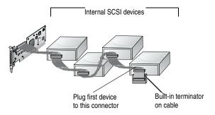
NOTE Internal Ultra2 and Ultra160 SCSI devices come from the factory with termination disabled and cannot be changed. Proper SCSI bus termination is provided by the terminator at the end of the LVD SCSI cable.
