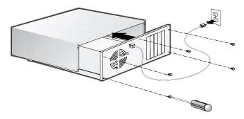
Locate an unused 64-bit PCI expansion slot and remove the expansion slot cover. If the computer does not have a 64-bit slot, you can install the card in a 32-bit PCI slot.
