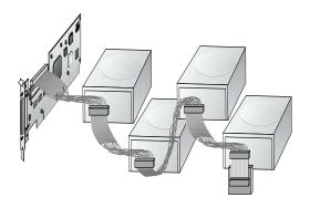
Plug the internal devices to the other cable connectors, starting with the connector at the terminated end of the cable.
