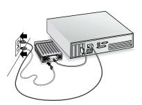
CAUTION Using a single-ended terminator will cause the SCSI bus to run in single-ended mode. LVD termination must be used to obtain Ultra2 transfer rates.
