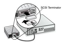
If you are installing only one external device, terminate the device and skip to Step 4.
