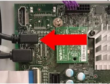
Locate the USB cable with the micro USB, the one in the top
