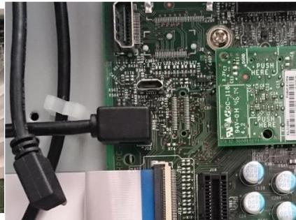
Unplug the top USB cable from the micro USB board connector.
