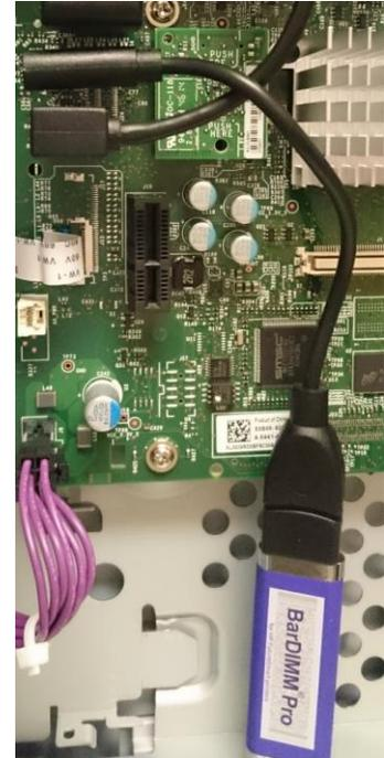
Connect the BarDIMM Pro cable to the board micro USB plug.
