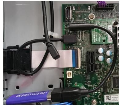
Connect the BarDIMM Pro cable to the board micro USB plug.
