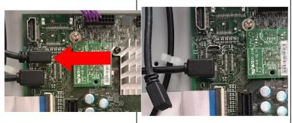
Locate the USB cable with the micro USB, the one in the top
