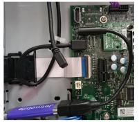
Connect the BarDIMM Pro cable to the board micro USB plug. Close the formatter, put the power cable back and switch on the printer.
