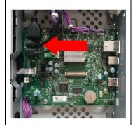
Locate the USB cable with the micro USB, the one in the center
