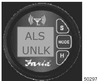
Alarm system unlocked
