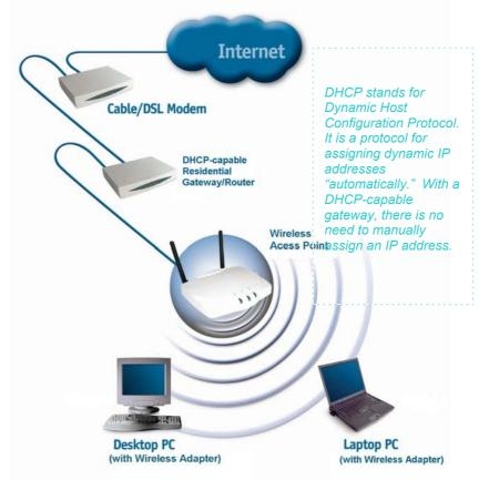
**Requirements:** A Residential Gateway/Router connected with an Ethernet (CAT5) cable to an 802.11g Access Point.
