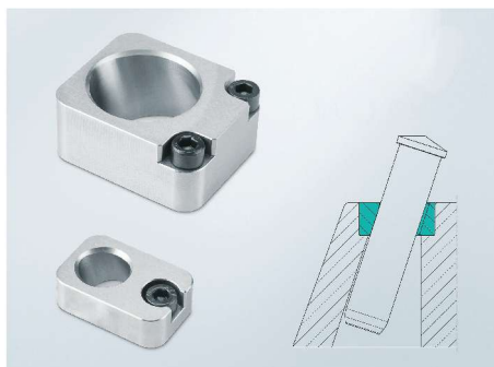
New guide for inclined pin from Meusburger simplifies machining, allows for stroke adjustment, and absorbs high force through maximum contact between guide and pin.
