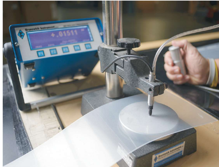
Impact Plastics prides itself on its ability to maintain tight tolerances of thin-gauge film, as evidenced by this off-line reading.
