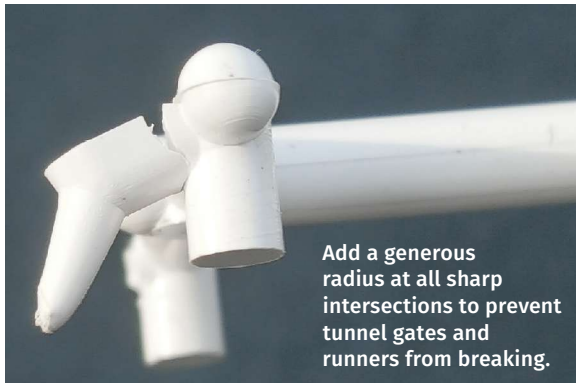
Using two ejector pins equidistant from a tunnel gate helps reduce the possibility of the gate breaking off.
