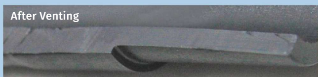
FIG 1 If air is not vented from the mold, it will cause inadequate filling, resulting defects that include short shots, poorly packed-out parts, burning of the plastic, voids in the parts, and dimensional variations.
