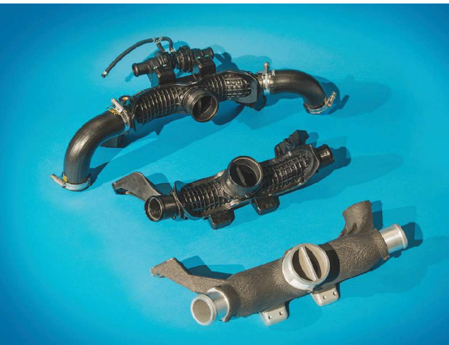
Heat-stabilized, glass-reinforced nylon 66 turbocharger outlet T-joint achieves a 42% weight savings and 35% cost reduction.
