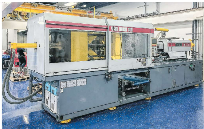
This 300-ton 1996 toggle press was tested with the new oil in an environmentally controlled lab where the machine's power factor is isolated from that of other equipment.
