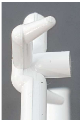
For shallow parts, stepping the parting line will allow you to use a larger tunnel-gate angle.
