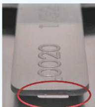
Tab Thickness = 0.03125 in. Vent Depth = 0.0020 in. Evidence of Flash
