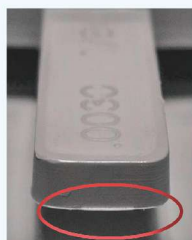
Tab Thickness = 0.125 in. Vent Depth = 0.0030 in. Evidence of Flash
