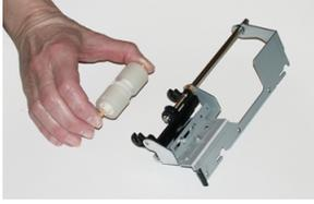
9. Replace a new retard roll into the black notches of the assembly using the same technique.
