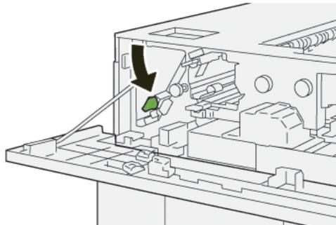
5. Open lever **2a** downward (①) and remove jammed paper (②).
