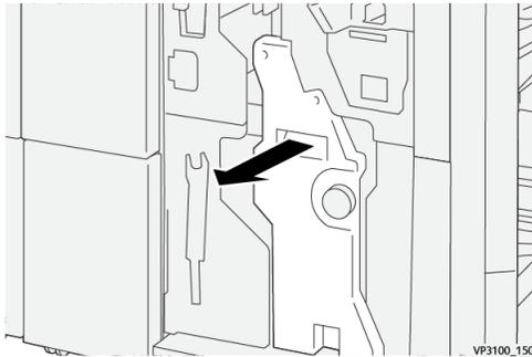
3. While holding the tabs on the staple cartridge, pull out the cartridge to remove it.
