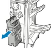
3. To remove the staple cartridge from the booklet maker, push down on the staple cartridge handle as shown, then pull the cartridge out and up.
