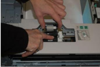
4. Replace the new roll by squeezing both ends of the metal shaft, and pushing down on the black tab, insert and release the roll ends into the notches.
