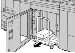
5. Remove the securing bar.
