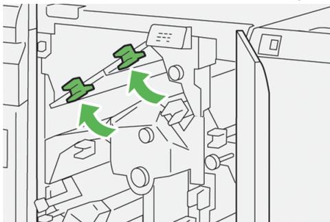
6. If you have difficulty removing any paper jams, open lever **1d** upward (①) and lever **2a** to the left (②).
