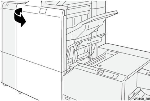
4. Rotate the knob **3b** to the right, and then remove the jammed paper.
