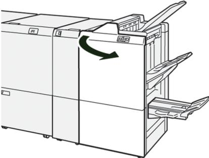
2. Open lever 3a to the left (1) and remove the jammed paper (2).
