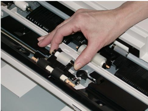
5. Remove and replace the retard roll using the same technique.
