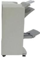
The BR Finisher with the optional Booklet Maker supports hole punching, stapling, and booklet making. The Right Top Tray is used for stacked output, and can receive up to 500 sheets of paper. The Right Center Tray is used for offset and/or stapled output and can hold up to 1,500 sheets. Both trays can be used for hole punched output (optional). The Bottom Finisher Tray is used for receiving saddle-stapled booklets.
