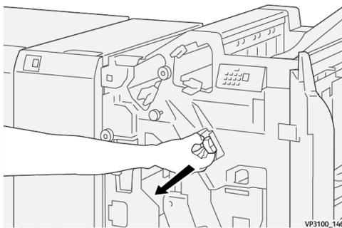
3. Holding the staple cartridge at the position indicated by the arrow, remove it from the unit.
