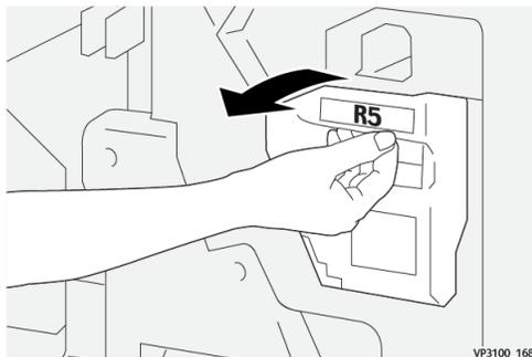
4. Place the used staple waste container into the supplied plastic bag.
