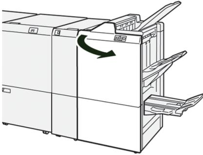
2. Open lever 1a to the left (①) and remove the jammed paper (②).
