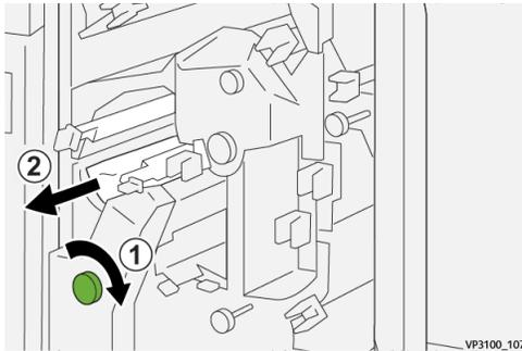
4. If you have difficulty removing the jammed sheet, grasp the top edge at the inner-right side of the sheet, and gently pull out the sheet to remove it.
