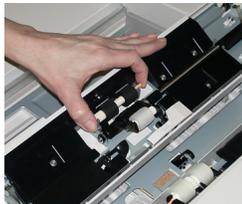
4. Remove and replace the nudger roll using the same technique.
