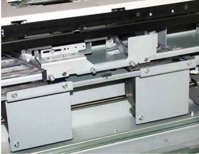
11. Screw in the 3 thumbscrews to attach the assembly. Do not over tighten.
