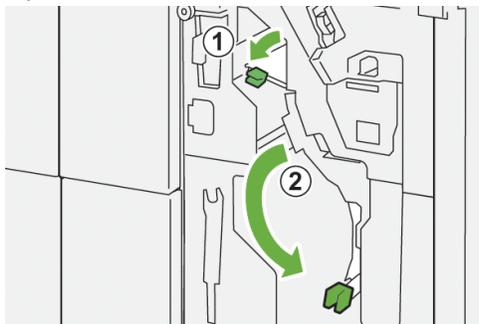
b) Rotate knob **1b** clockwise (①) and remove the jammed paper (②).
