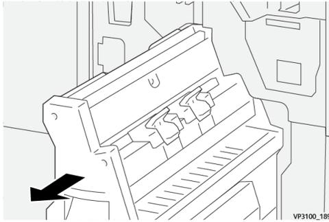
3. Rotate knob **3b** counterclockwise (①) and remove the jammed paper (②).
