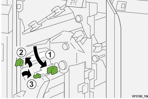
3. Rotate knob **2f** clockwise (①) and remove jammed paper (②).
