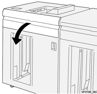
2. Open lever **2a** downward (①) and remove jammed papers (②).
