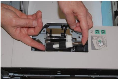
8. Finally, replace the retard roll. Squeeze the orange shafts of the retard roll and lift out of the assembly.
