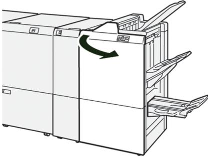
2. Open lever 1c to the right (1) and rotate knob 1e clockwise (2). Remove the jammed paper (3).
