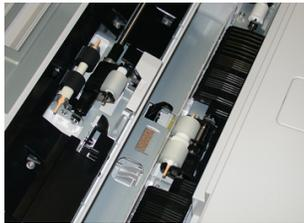
3. Remove and replace the feed roll by squeezing the metal shaft and lifting out.
