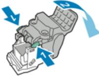
6. To remove the staple refill, press the rear of the refill container as shown.
