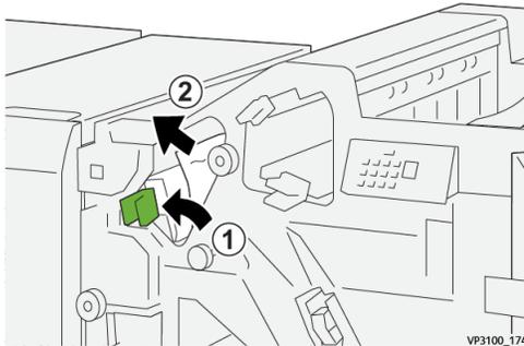
3. If you have difficulty removing any paper jams, rotate knob 1b clockwise (①) and remove the jammed paper (②).
