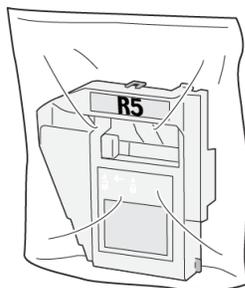
5. Insert the new staple waste container by lowering it into position and gently pushing it into place.
