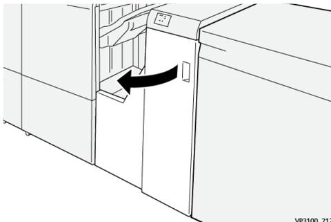
2. Open level 1 downward and remove the jammed paper.
