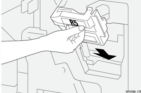
6. Move the lock lever under R5 toward the right to the closed-lock mark.
