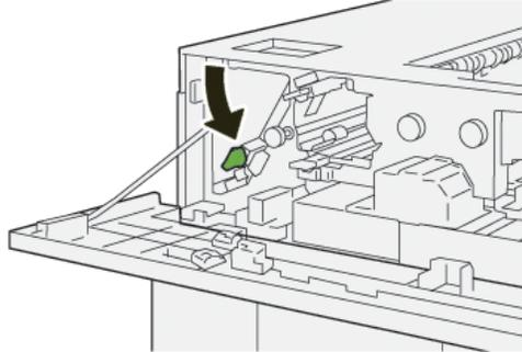
4. Open lever **2b** upward (①) and turn knob **2c** counterclockwise (②); remove jammed papers (③).
