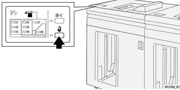
2. Make sure the HCS front door is unlocked and then open it.
