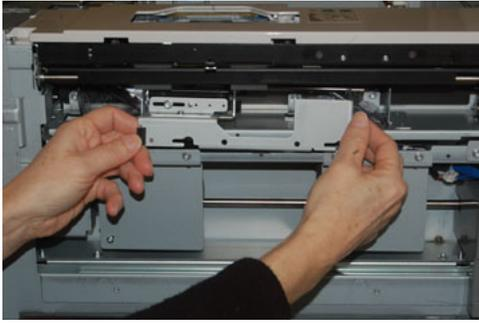
7. With the retard assembly out, access and remove the feed roll. To remove, squeeze both ends of the metal shaft and lift out. To replace, squeeze both ends of the new roll shaft, and insert and release the roll ends into the notches.
