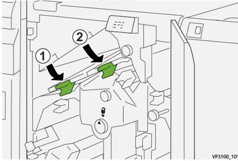
4. Turn knob **1c** clockwise (①) and remove jammed papers (②).
