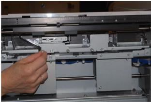
6. Slide the retard assembly all the way to the left so it is out of the slots. Pull the assembly out towards you until completely removed from the tray. Set aside.
