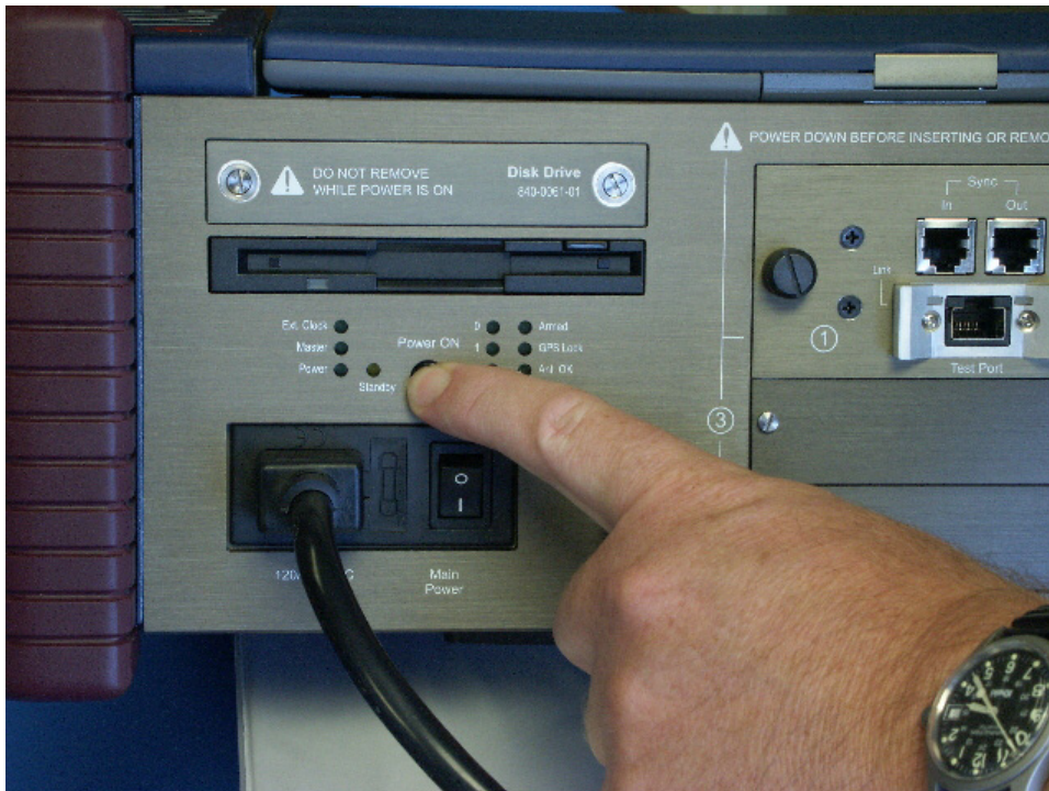
Figure 12-8. IXIA 250 Standby Switch
