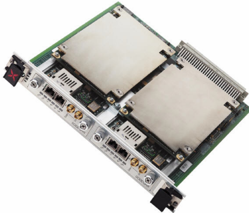
Figure 26-1. LM622MR Load Module with Pluggable PHYs Installed
