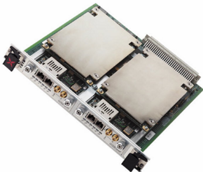
Figure: LM622MR Load Module with Pluggable PHYs Installed
