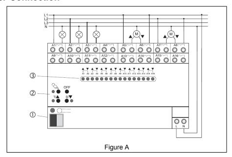
The bus line is connected to the bus connecting terminal (1).
