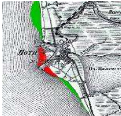
Figure 2. Heavily Eroded Sections of the Coast Line (1906-1980)
