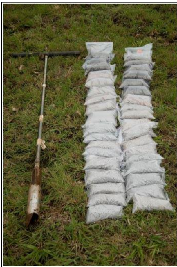
Figure 8: A soil auger (left) with soil samples collected in zip lock bags lined up next to it.
