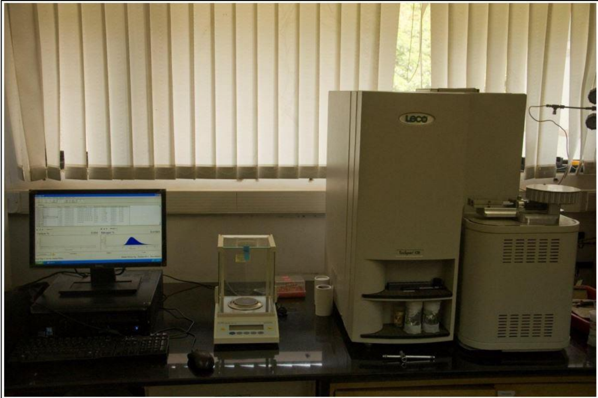
Figure 9: LECO Corporation's TruSpec Micro used for analyzing soil samples to find their carbon and nitrogen content.
