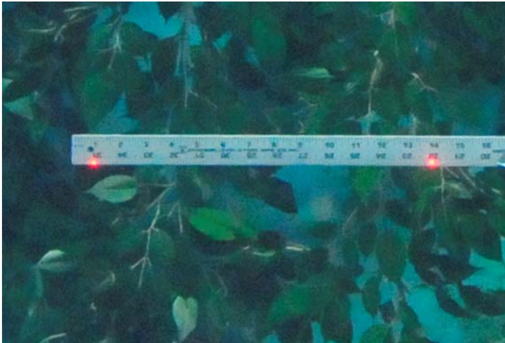
Figure 5. Laser spots set 13” apart filmed through 14 feet of water (enlarged and cropped).
