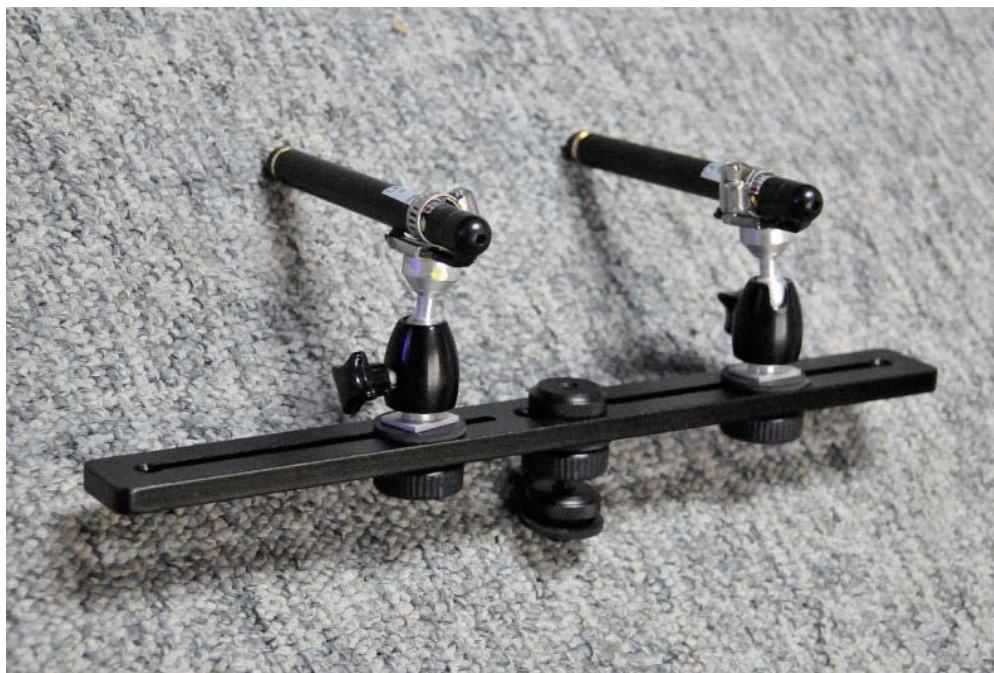
Figure 2. Laser measuring system using inexpensive laser pointers.
