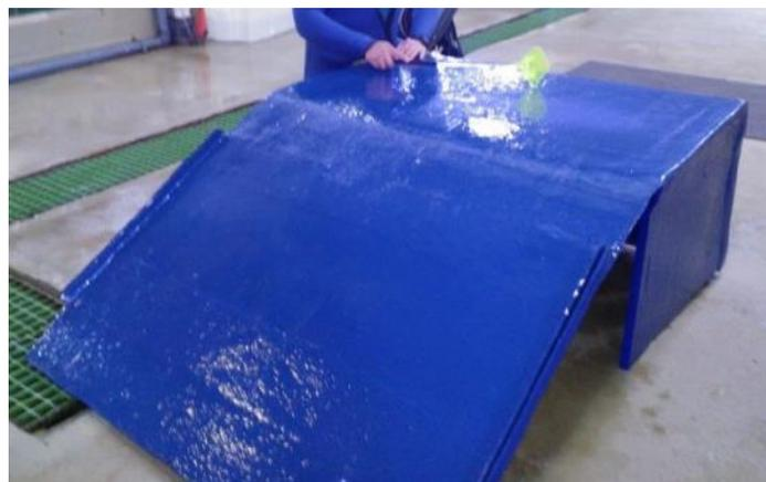
**Figure 1:** The fiberglass ramp and platform, seen out of water in association with the acrylic target.
