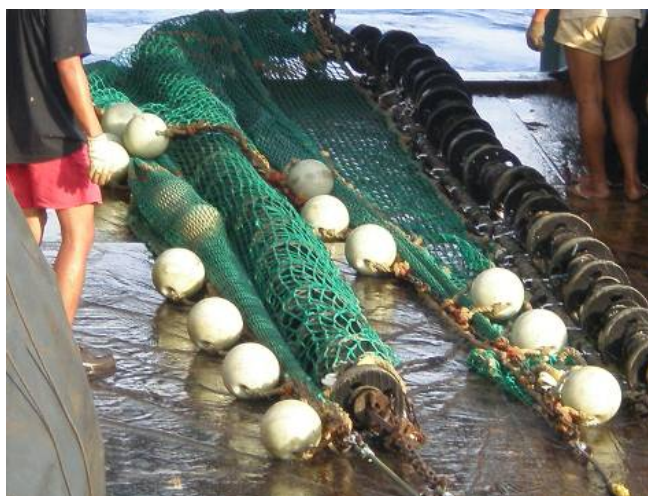
Otter trawl used on board MV DA-BFAR for AURORA 2007 expedition
