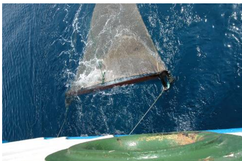
Beam trawl used on board MV DA-BFAR for AURORA 2007 expedition
