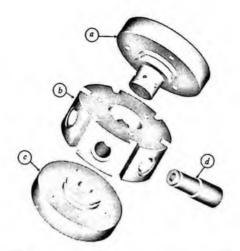
Figure 1. Rendering of the components of the measurement chamber; a) flow splitter; b) body; c) cap; d) connector.
