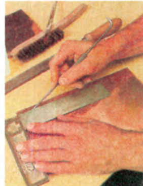
4 Scribing lines or circles on metal surfaces
