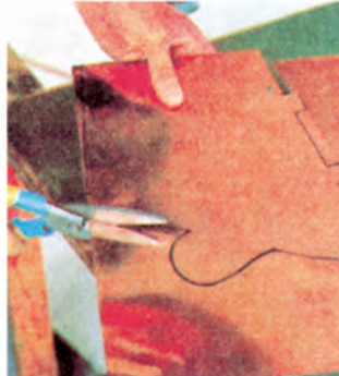
15 Shearing thin sheets of metal
