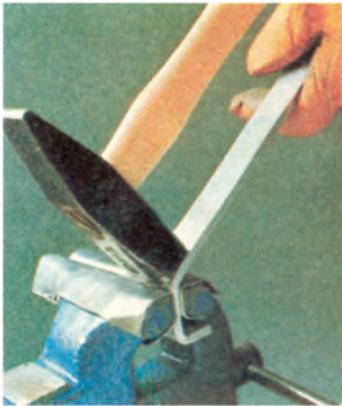
10 Bending metal sheets
