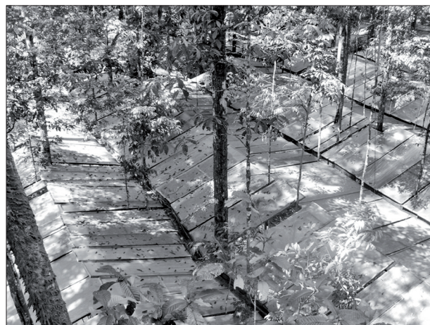
Figure 2. Part of 6,000 transparent plastic panels established in the experimental plot. Photo: L. V. Ferreira.
